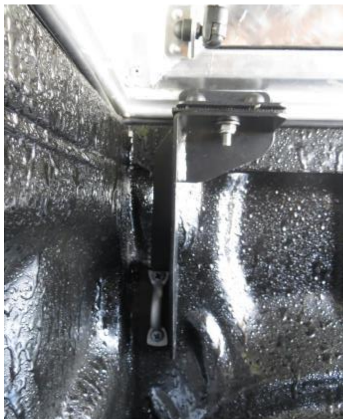
Figure 21: Front-Right Support Bracket Installed
